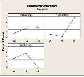
Fig.1: Effects of Process Parameters on MRR
